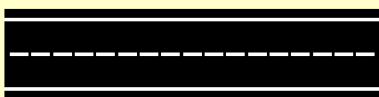
Border or edge lines. Continuous lines at the edge of mark the limits of which a road user can safely use.
